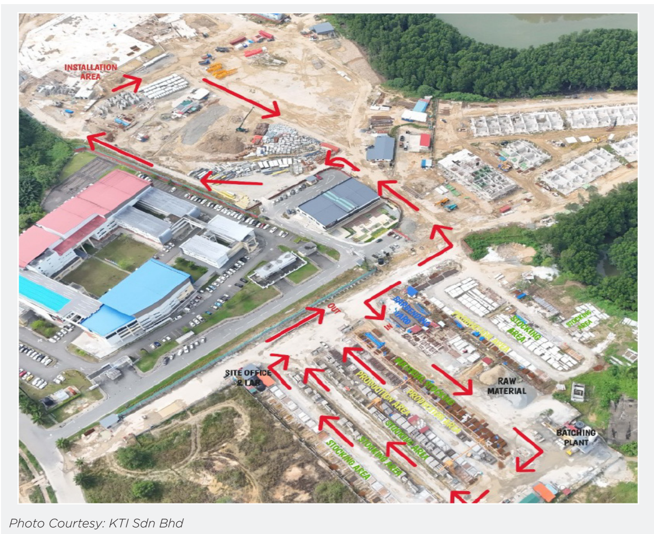
Temporary precast concrete casting yard layout:
